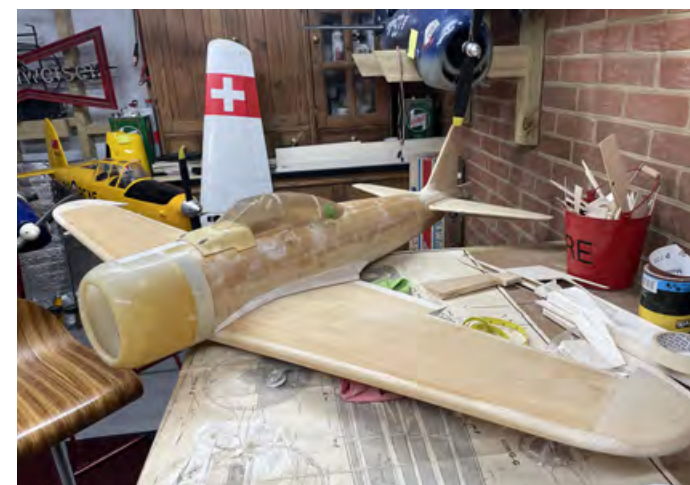
Wing root fairings made from balsa
