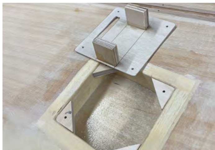
Servo boxes constructed and let into the foam wing
