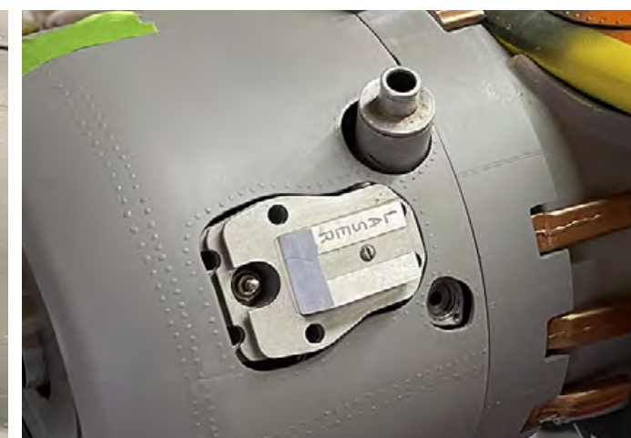
Cowl neatly cut for Laser 100. Note rivets!
