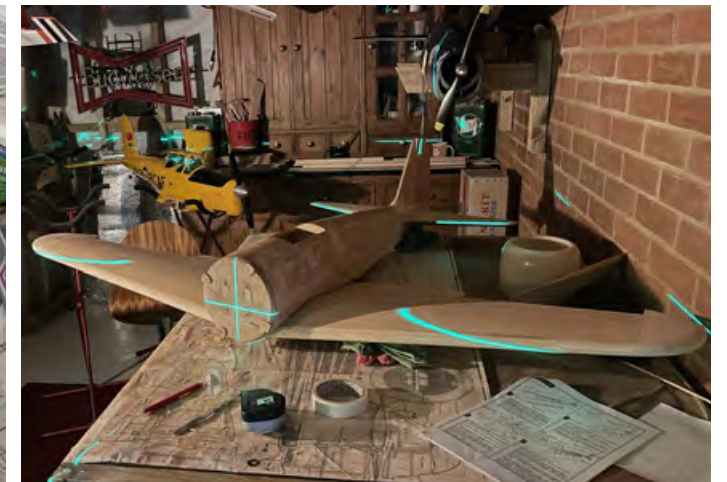
Checking alignment with laser
