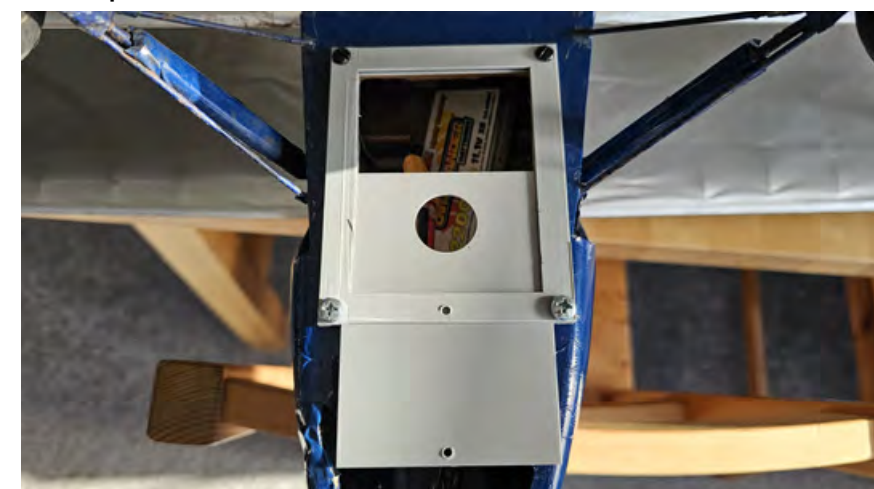
Sliding battery hatch in action
