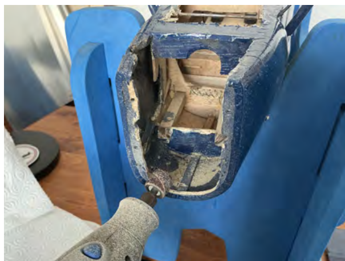
Using Dremel to clean out the nose area
