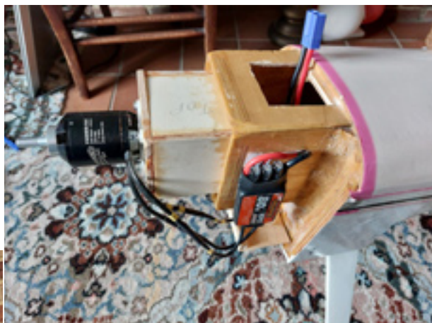
Right: Overlander 500kV motor fitted to Giles. Photo: Les Crane Below: Ivan takes the sticks for taxi trials! Photo: Grahame Pearson
