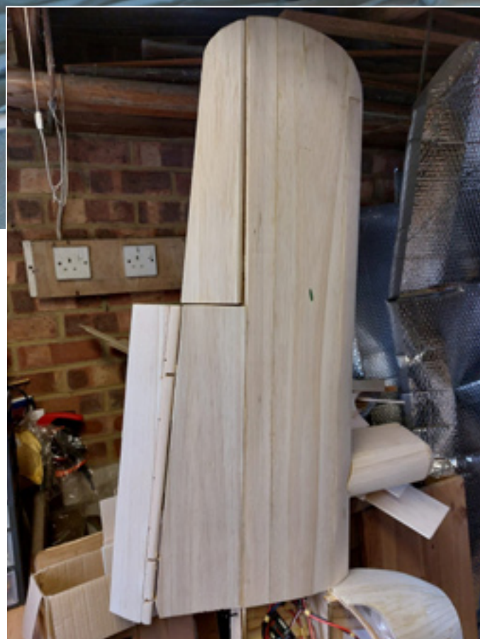
Above: Miles Gemini now fully planked. Left: Aileron and flap loosely fitted. Photos: Les Crane
