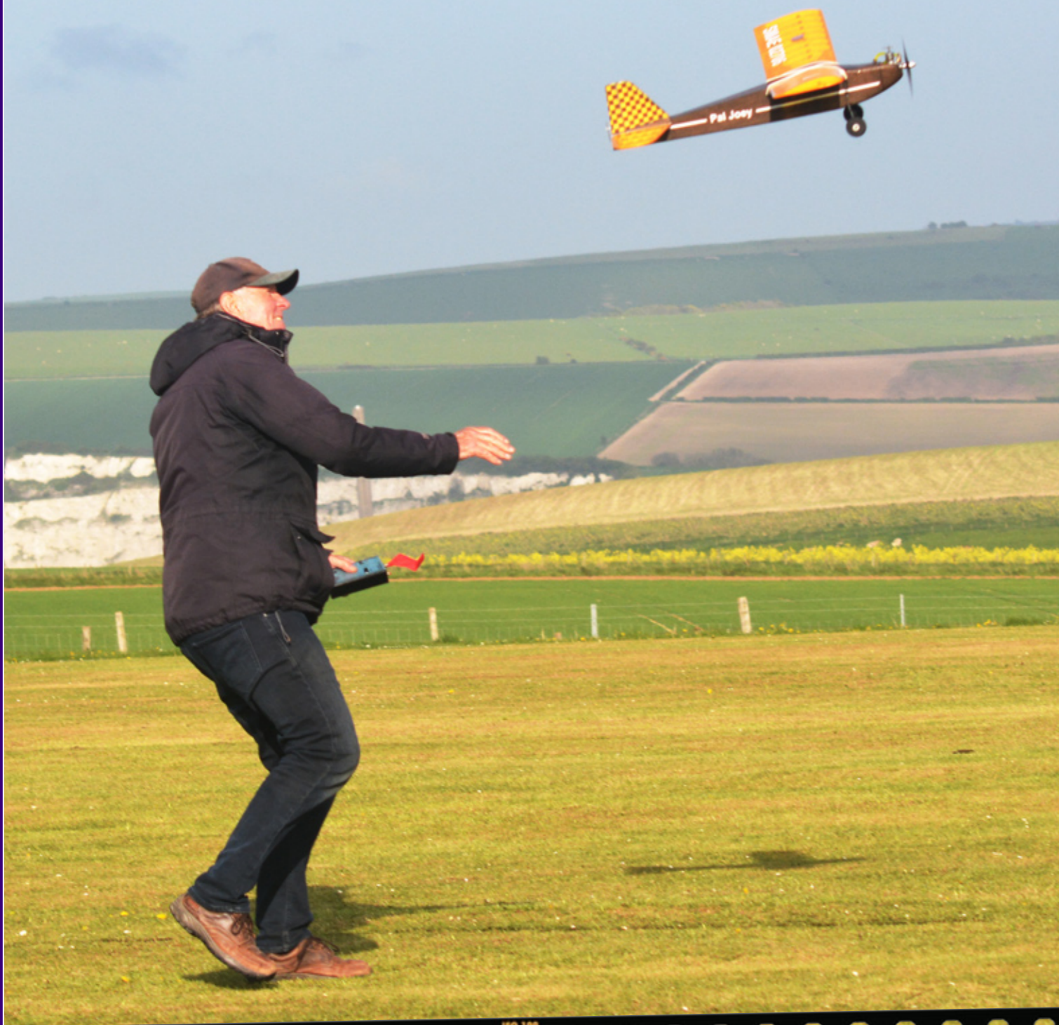
Chairman Derek's Pal Joey powered by a PAW 1cc diesel and controlled by single-channel (rudder only) radio – real old time stuff
