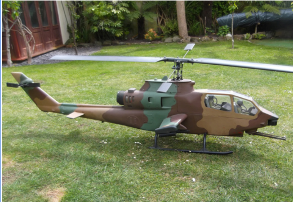
Jerry Hansen's 700-size Cobra scale helicopter with a 38cc petrol engine. All photos: Jerry Hansen
