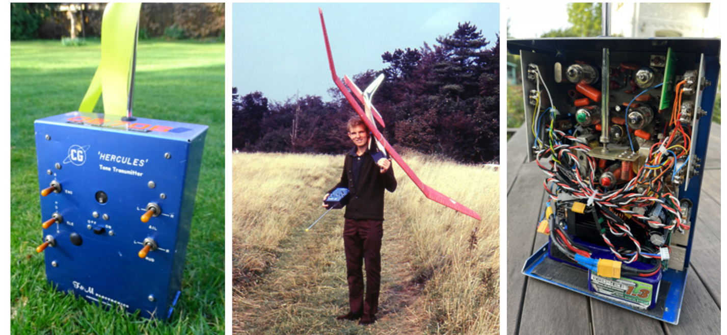
Derek Woodley’s unnamed 9 foot wingspan own design glider was built by Derek in 1964 and restored during COVID lockdown, seen in the top two photos flying again in 2022. The centre photo, above, shows Derek in 1964 with the same model. It was flown with a then-state-of-the-art F&M Hercules 10 channel 5-valve transmitter operating on 27Mhz that required three batteries: two 67.5V and one 1.5V dry cell. The receiver is an F&M Midas transistorised 10 channel reed superhet running on a 7.2V NiCad battery. This equipment was manufactured in the USA and imported by Harry Brooks. Harry was using this gear when he was joint winner of the 1963(?) World Championships, held in the UK. There was no comparable equipment manufactured anywhere in Europe at that time. Above photos, left and right: Amazingly Derek still flies the glider with the same 27Mhz radio gear, albeit modified to run on modern LiPo batteries!
