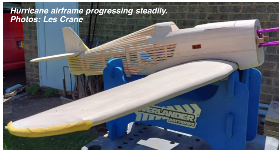
Control surfaces fabric covered – as per full-size
