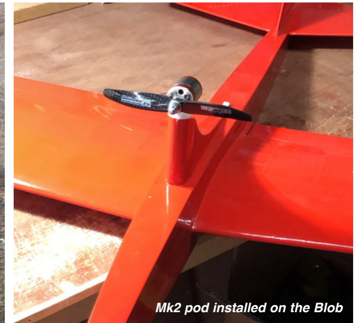
Mk2 pod with improved aluminium motor mount but with motor fixed in position
